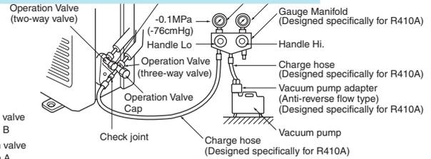
Securely tighten the operation valve cap and the check joint blind nut after adjustment.
