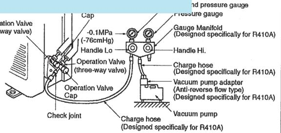
Securely tighten the operation valve cap and the check joint blind nut after adjustment.
