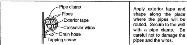
Apply exterior tape and shape along the place where the pipes will be routed. Secure to the wall with a pipe clamp. Be careful not to damage the pipes and the wires.
