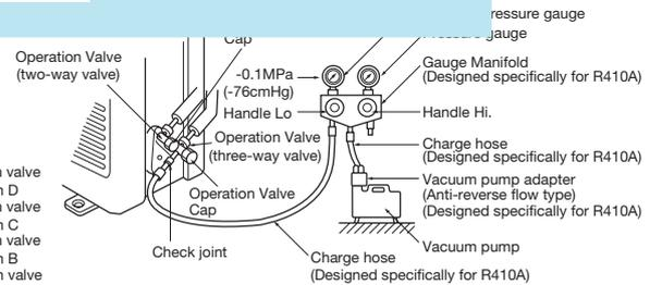
Securely tighten the operation valve cap and the check joint blind nut after adjustment.
